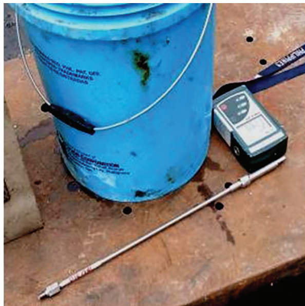
Figure 2. The bare source rod containing the Cf-252 sources. The active part is in contact with the dose rate meter.
