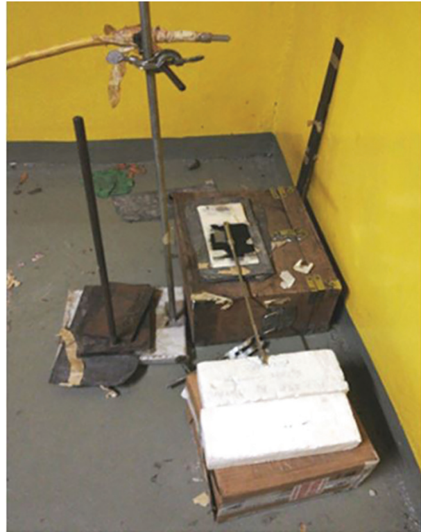
Figure 6. The radiographic set-up showing the guide tube where the Ir-192 source is located and the source rod laid bare on top of the film.
