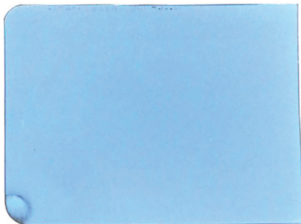
Figure 3. The underexposed radiograph in clear light blue acetate indicates less radiation interaction with silver halide crystals.
