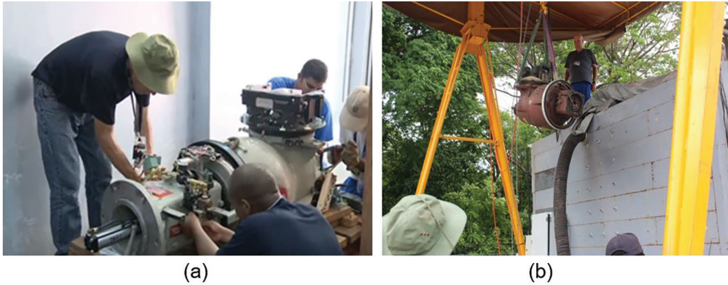
Figure 3. a) Dismantling before subjecting the device to the MHC; b) pre-dismantled teletherapy device being lowered on the cavity of the MHC.
