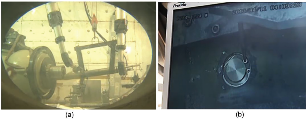
Figure 4. a) Source drawer being retrieved inside the teletherapy device; b) removal of the source from the drawer as viewed from one of the cameras inside the MHC.
