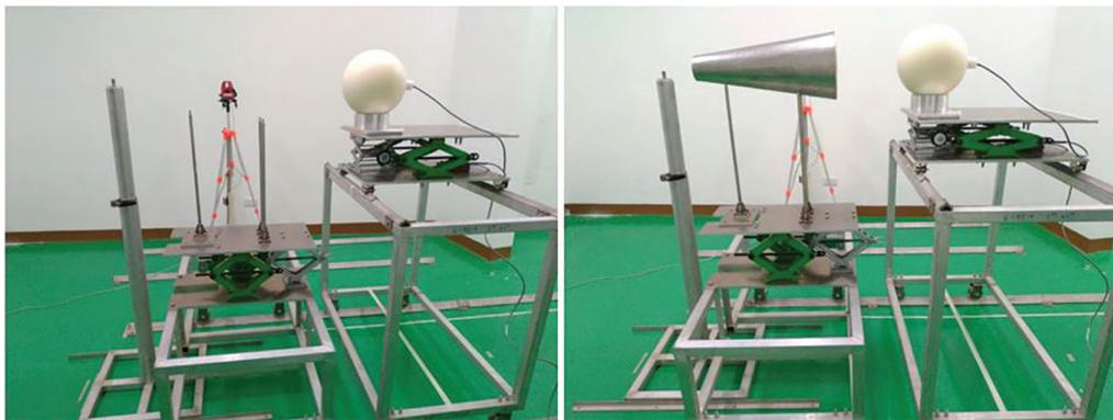
Figure 2. Actual experimental set up using the dummy neutron source, without the shadow cone (L) and with the shadow cone (R), and the spherical proportional counter inside the Bonner sphere.
