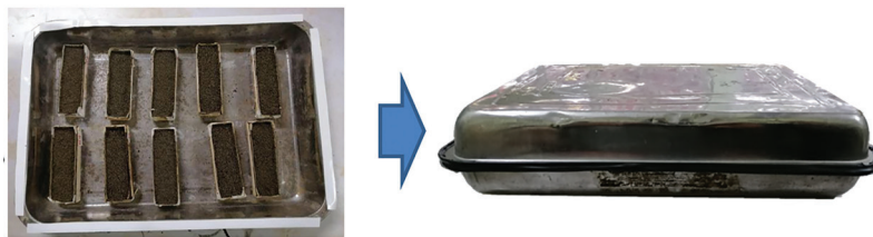
Figure II. Metallic chamber as an enclosure for heating geconcrete cast.
