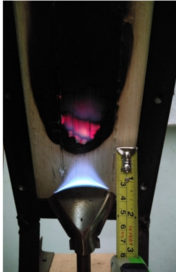
Figure 1. Fire testing setup with the height of flame maintained in the range of 25.4–38.1 mm.
