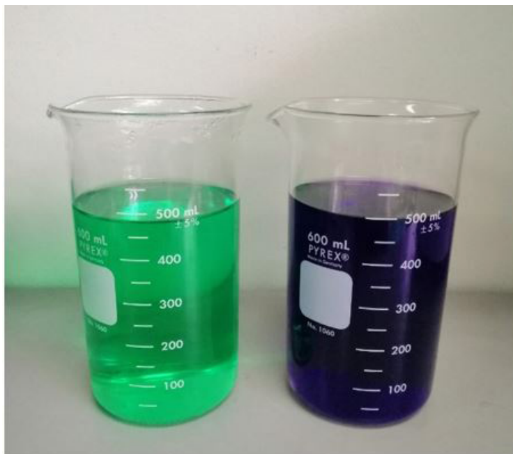
Figure A1. Ethaline-nickel chloride electrolyte (left) and ethaline-nickel chloride-ethylenediamine plating bath (right).
