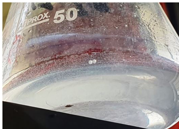
Figure 6. Formation of white precipitate and aggregate on agitation of an aqueous solution of lead with extracted EPS of Lysinibacillus sp. SS1.
