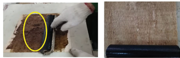
Figure 6. N-100m (left) shows the agglomerated TSP (yellow oval) with glue spreading difficulty causing uneven glue spread. N-200m (right) showing uniform and even spread of the glue-mix with TSP.
