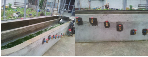
Figure 6. Sampling ports of the oval raceway pond at different heights.
