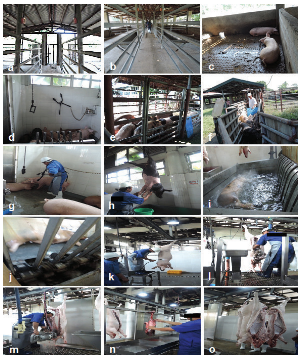
Figure 1. Facility and operation at the visited semi-automated and semi-mechanized slaughterhouse (SH1): (a) receiving/off-loading area, (b) passageway to lairage area, (c) holding pen in lairage area, (d) stunning area, (e) showering of pigs, (f) driving pigs to slaughter area, (g) stunning, (h) sticking/bleeding, (i) scalding, (j) dehairing, (k) singeing, (l) evisceration, (m) splitting into half, (n) meat inspection, and (o) washing and hanging of carcass.
