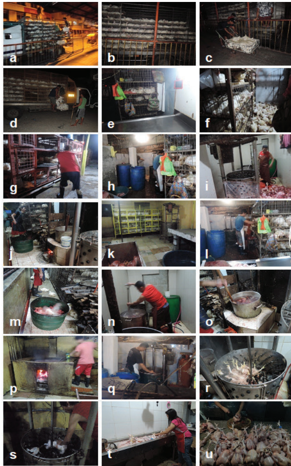
Figure 3. Facility and operation at the visited poultry dressing plants (PDP1, PDP2, PDP3, and PDP4): (a–b) transportation vehicle of live animals and unloading of chicken, (c–d) transfer of chickens from vehicle to holding area, (e–g) holding area, (h–k) slaughtering area, (l–m) sticking and bleeding, (n–p) scalding, (q–s) defeathering, and (t–u) evisceration.
