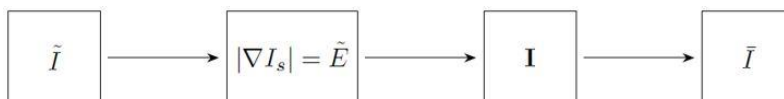
Figure 2. Flow of the three-step approach where \tilde{I} is the given image, I_s is the smooth approximation, \tilde{E} is the fuzzy edge map, I is the binary edge map, and \hat{I} is the post-process binary edge map.
