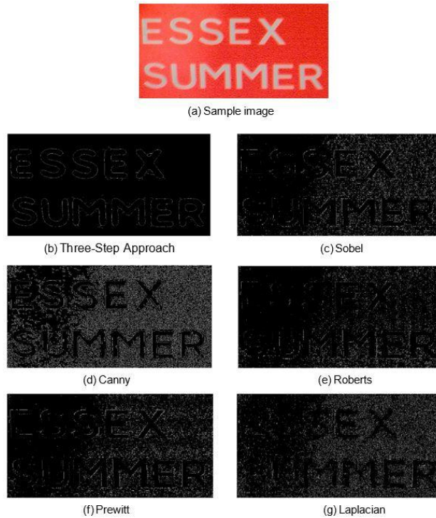
Figure 12. The three-step approach, with \alpha = 5 \times 10^{-3} , and other edge detection methods applied to sample image (a) from (Mosleh et al. 2012).
