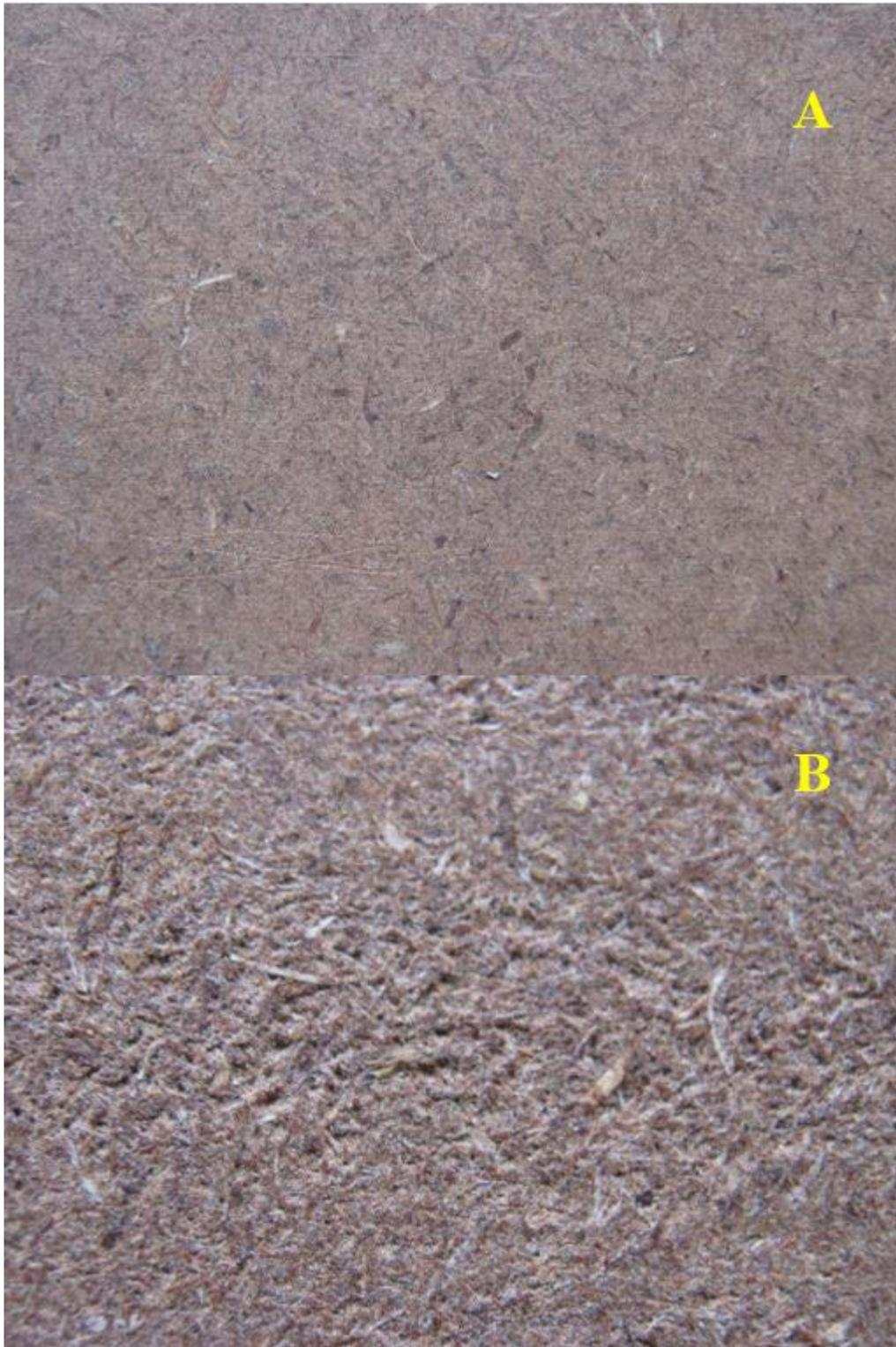
**Fig. 6.** Surface appearance of the MDF specimens (A) before the ice-blasting, and (B) after the ice-blasting, showing severe abrading effects.
