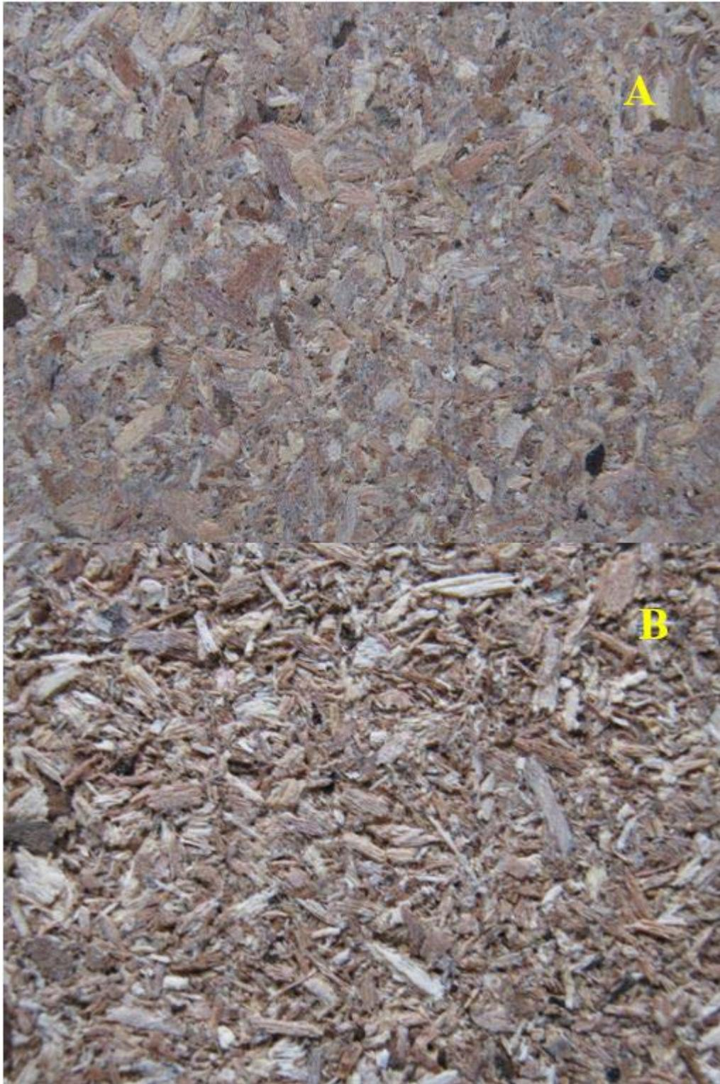
**Figure 7.** Surface appearance of the particleboard specimens (A) before the ice-blasting, and (B) after the ice-blasting, showing severe abrading effects.
