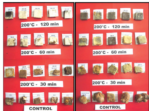
Figure 4. Comparison of the damaged sustained by the treated and control samples after exposure to Fomes lividus (left) and Lenzites striata (right) at 200° C for 30 to 120 min.
