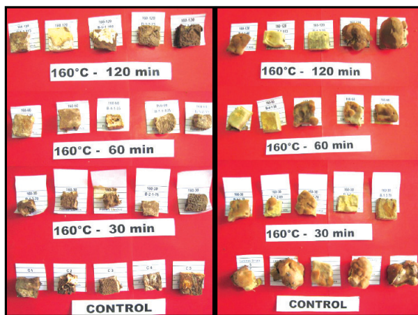
Figure 2. Comparison of the damaged sustained by the treated and control samples after exposure to Fomes lividus (left) and Lenzites striata (right) at 160° C for 30 to 120 min.
