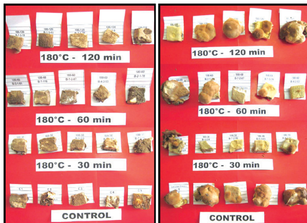
Figure 3. Comparison of the damaged sustained by the treated and control samples after exposure to Fomes lividus (left) and Lenzites striata (right) at 180° C for 30 to 120 min.
