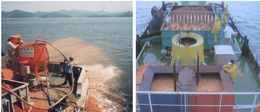
Figure 5. Harmful Algal Blooms control by Clay dispenser (left) and electrolytic clay dispenser (right) in Korea.
