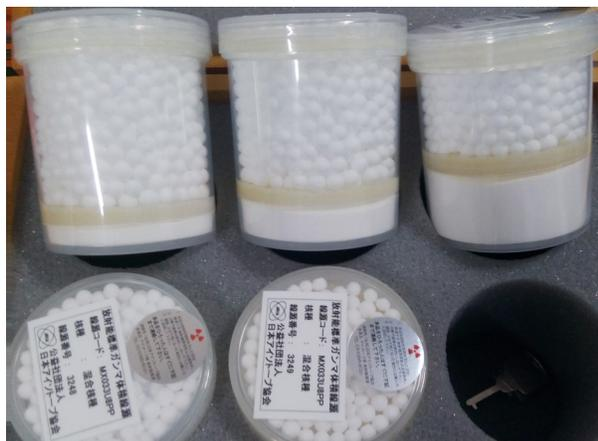
**Figure 2.** Mixed efficiency standards made from Al<sub>2</sub>O<sub>3</sub> with heights of 0.5, 1, 2, 3, and 5 cm to address the issue on geometry made by the Japan Radioisotope Association.
