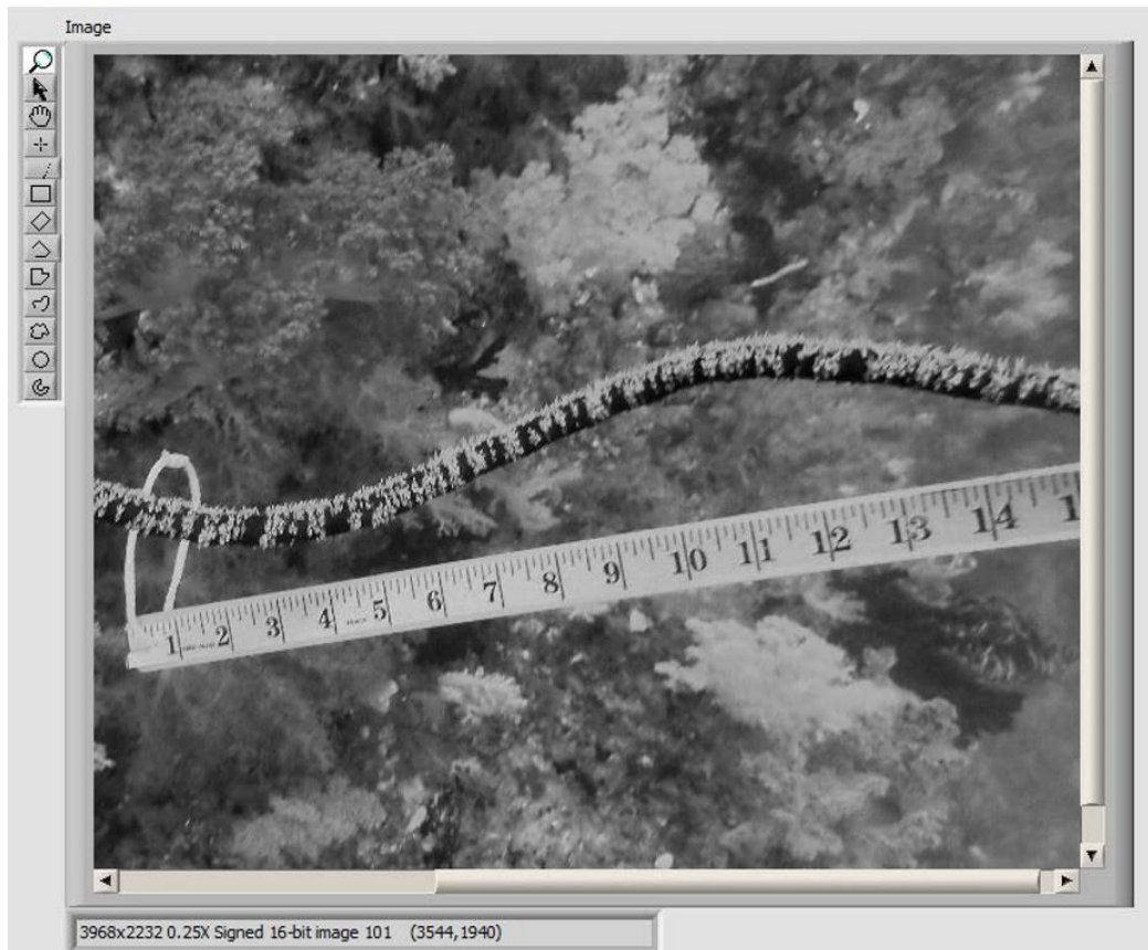
Figure 2. A sample image of a black coral. A measuring tape was used as a scale bar and was needed during image analysis using LABView.
